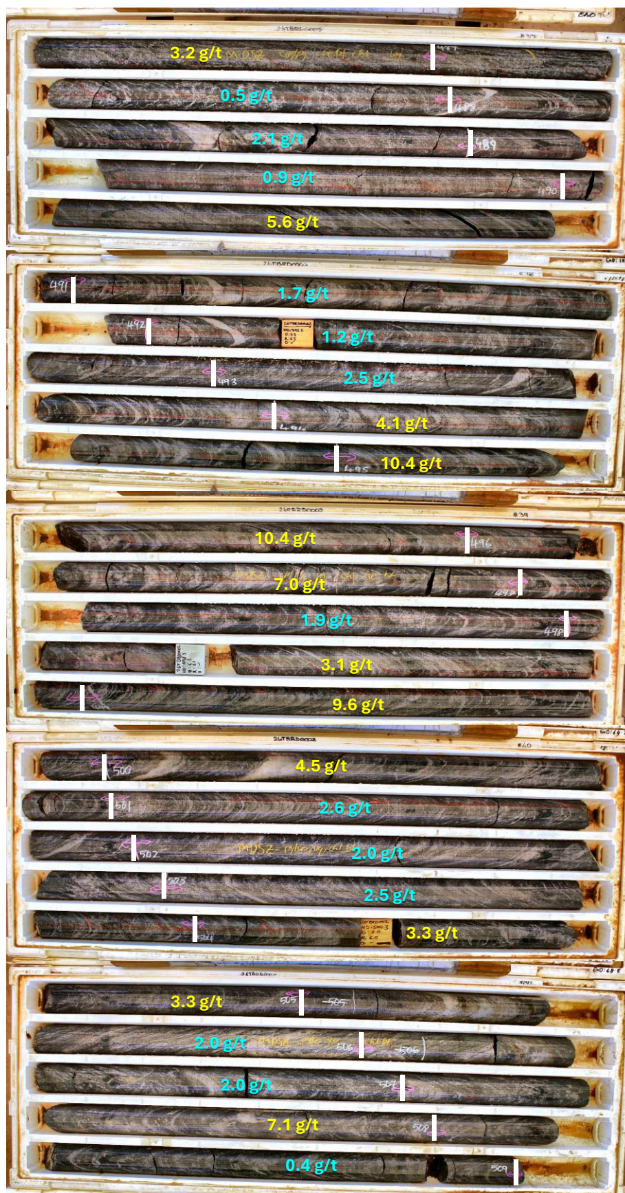
Figure 4: Diamond drill core showing shearing and mineralisation in hole 26TBRD002 from 486m downhole.
