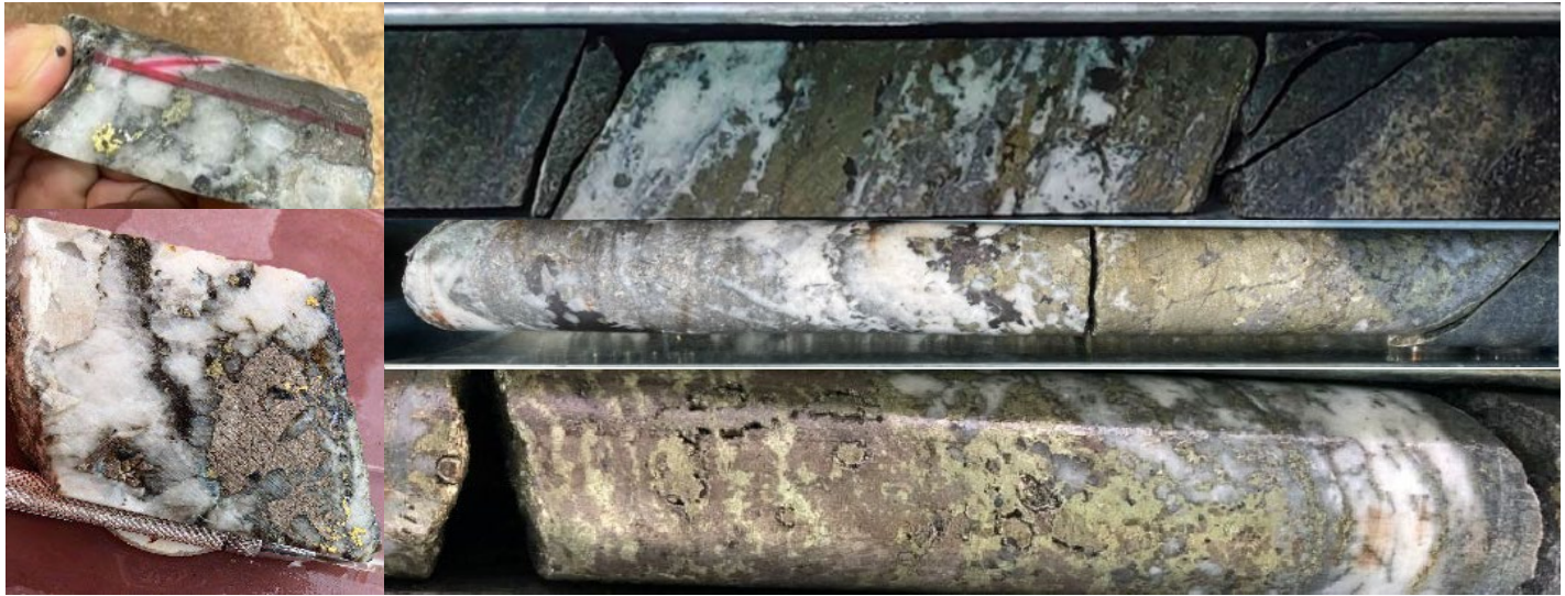
Figure 9 | Mineralised veins in Memot diamond core. Quartz veining with Pyrite, Arsenopyrite, Pyrrhotite, Chalcopyrite and Sphalerite sulphides. In order from Left hand Side photos: DD24MMT243 - 1m @ 2,090.00g/t Au from 130m. Right Hand Side Top to Bottom DD21MMT001 - 1m @ 8.91g/t Au, 2.16% Cu from 48m, DD22MMT013 - 0.4m @ 17.70g/t Au, 230g/t Ag, 2.78% Cu, 0.56% Pb and 1.74% Zn from 190m and DD21MMT006 - 1m @ 25.4g/t Au, 73g/t Ag, 1.81% Cu, 0.1% Zn from 30m
