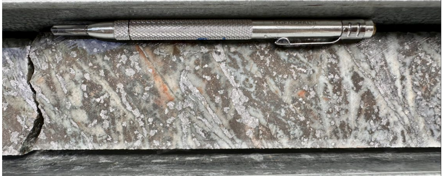
Figure 19 | Mineralised vein in RCDD26OKV824W1 at approximately 530.5m downhole depth. The vein comprises predominantly euhedral arsenopyrite associated with quartz carbonate veins within a hornfelsed sedimentary host. The photograph shows approximately 20cm of core from within the intercept of 78.80g/t Au from 530–531m
