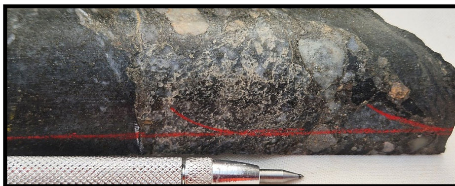
Figure 4. Pebble dyke with clasts of quartz vein and silica with pyrite ± bornite that are sourced from a deeper level and milled by the hydrothermal brecciation (PHD084 at 1582.7m).
