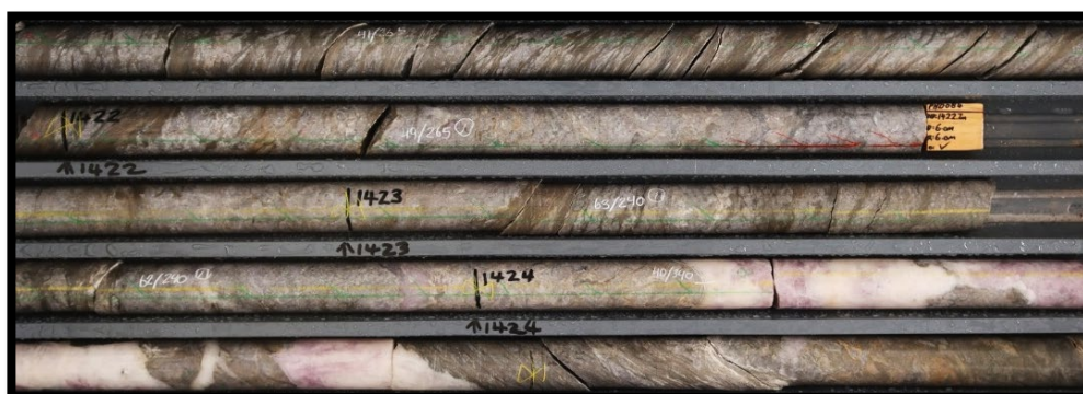
Figure 3. White and pink anhydrite ± chalcopyrite veins (magmatic derived fluids) that crosscut the earlier advanced argillic pyrophyllite-silica-pyrite alteration (PHD084 from 1421m).
